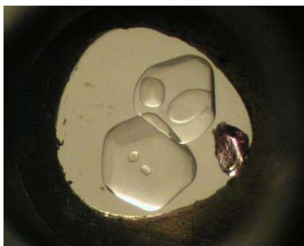
Figure 1. Standard microscope image of ice crystals in liquid water, at a pressure of 0.9 GPa and room temperature. A ruby chip is on the right side of the gasket hole.
